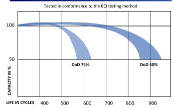
\* Cycle life is measured with a discharge current 0,2C, charged 16h and rest capacity of 2/3 Cn
